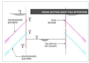
conditions were constantly changing along the length of the wall. The analysis therefore had to be done incrementally, taking design cross sections for each section of the tunnel. Modeling was performed using an effective stress analysis based on BS8002, using the analysis software ReWaRD. The design of the sheet pile system was performed in accordance with the requirements of BS5950. Anchors were designed based on BS8081, which is a working load design standard.
