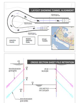
cheaper and technically sound solution. The proposed embedded steel sheet pile solution was adopted. Large parts of the retaining wall needed to be supported by one and/or two levels of ground anchors with a continuous waling beam.
