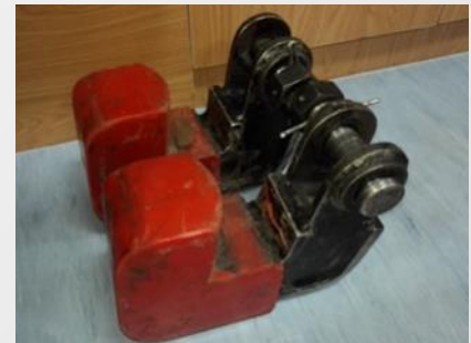
Customized lifting hooks used for lifting to prevent damage.
