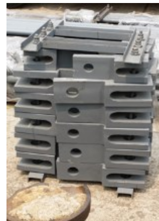
TIE ROD T-PLATES TO KING H PILES
