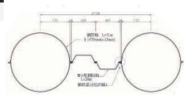
Figure 1 Plan view of the Combi wall profile
