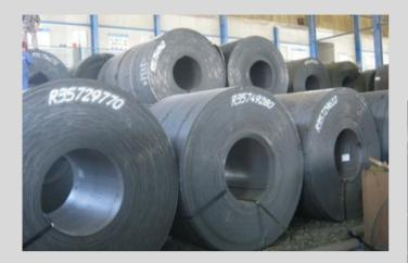
The quality of the raw material is critical to ensure the final product meets the project specification. Thickness of each coil is inspected and the identity of the material shall be traceable with each coil.
