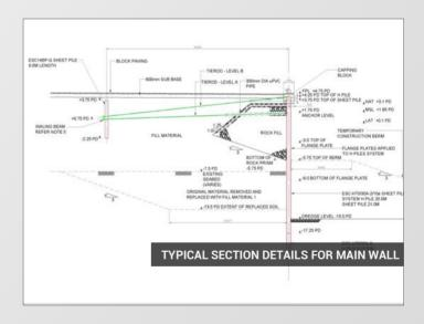
All calculations for structural capacity of the sheet pile systems were performed post corrosion loss.
