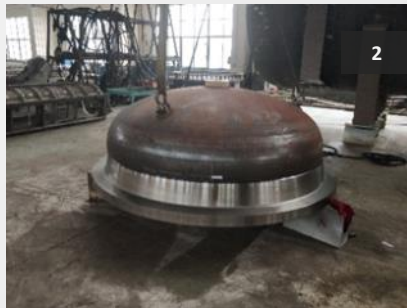
Picture 1 – Forming of Shaft Cap
