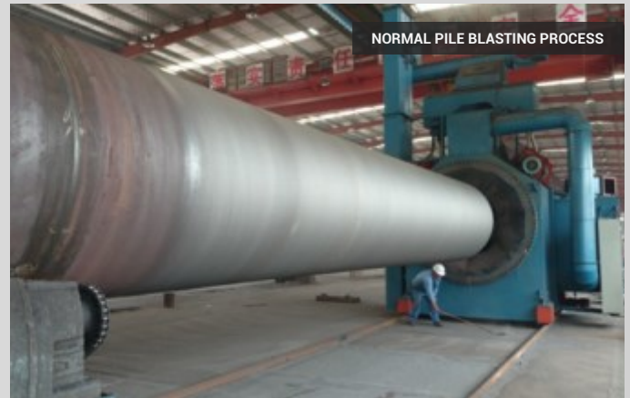
MONOPILE BLASTING PROCESS
