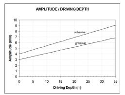
Figure 4. Required Amplitude
