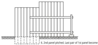
6. 2nd panel pitched. Last pair of 1st panel becom-1st pair of 2nd panel, gates supported by through bolting to last driven pair
