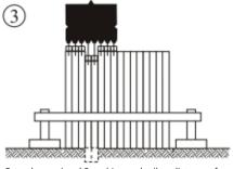
Extend rams 4 and 5 pushing each pile a distance of 750mm into the ground
