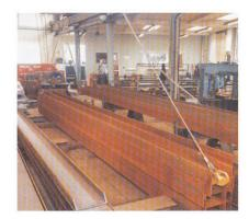
The Dawson Lifting Shoe is purpose designed for handling structural sections of steel in workshops, stockyards and on construction sites.
