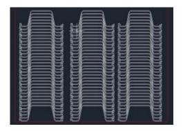
For Z shape sheet piles, the piles are typically stacked diagonally, with alternating connectors. This also makes driving more straightforward as the piles are progressively picked up from one side and are in the correct orientation.
