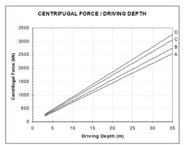
Figure 3. Required Centrifugal Force
