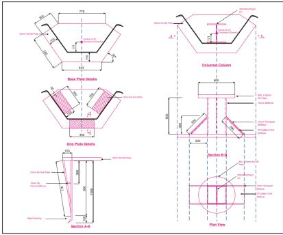
Special Driving Cap & Dolly for ESC Wide Profile Sheet Piles
