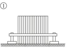
Pitch panel of sheet piles into guide beams supported on stable trestles
