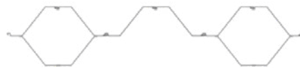
Box King Piles (fabricated out of 2 ESC-HRZ Piles & 1 Cold Formed U Pile)
