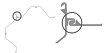
ESC-9E Hot Rolled Clutch Interlock (compatible with all ESC-HRZ Sheet Piles)
