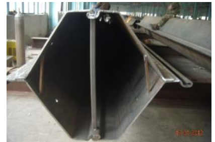
Box King Piles (fabricated out of 2 CRZ Piles & 1 Cold Formed U Pile)
