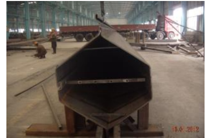
Box King Piles (fabricated out of 2 CRZ Piles & 1 Cold Formed U Pile)
