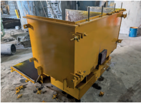
MOULDS FOR CONCRETE CASTING, UAE
