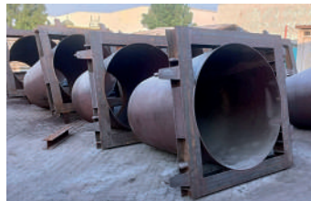
TREMIE PIPE FABRICATION
