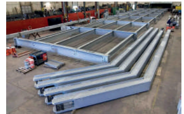
STRUCTURAL STEEL COLUMNS/BEAMS
